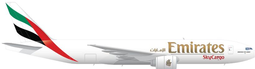
**BOEING 777F** Number of Aircraft: 7 Range: 9,260km Length: 63.7m Wingspan: 64.8m
