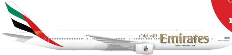
**BOEING 777-300ER** Number of Aircraft: 86 Capacity: 354-442 Range: 14,594km Length: 73.9m Wingspan: 64.8m
