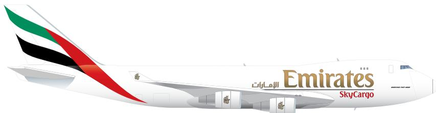
**BOEING 747-400F/747-400ERF** Number of Aircraft: 1/2 Range: 8,232km/9,204km Length: 70.6m Wingspan: 64.4m
