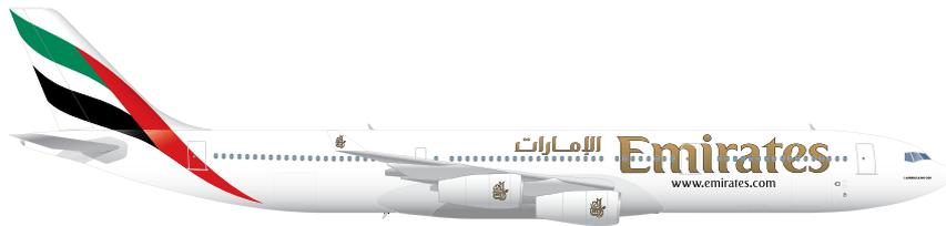
**AIRBUS A340-300** Number of Aircraft: 8 Capacity: 267 Range: 13,350km Length: 63.6m Wingspan: 60.3m
