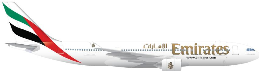
**AIRBUS A330-200** Number of Aircraft: 24 Capacity: 237-278 Range: 12,200km Length: 58.8m Wingspan: 60.3m
